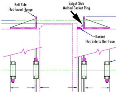
4. Install the gasket (Bevel Cut) on the spigot side of the joint with the flat side facing toward the pipe bell. For large or oversized cast iron pipe an additional gasket has been included to accommodate the pipe diameter. Gaskets may be cut to meet up. Follow original bevel angle to ensure complete match. Slide the gasket toward the joint so that flat side of the gasket meets up with the face of the bell.
