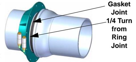
To ensure integrity of installation, wait 15 minutes, inspect for leaking, and confirm bolt torque. If necessary, loosen clamping bolts, tighten rod bolts evenly as required to stop the leak. Re-tighten clamping bolts.
