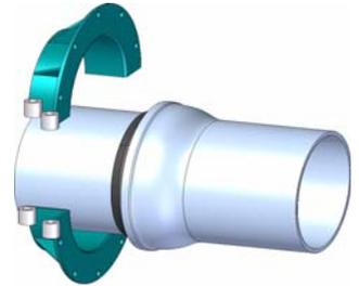
5. On the bell side of the joint install the second set of clamp ring segments in the same manner. Loosely bolt the segments together to allow movement. Complete installation by inserting the long rods through the segments and over the joint into the corresponding bolt holes of the opposite clamp rings. Loosely assemble nuts on the ends of the bolts.
